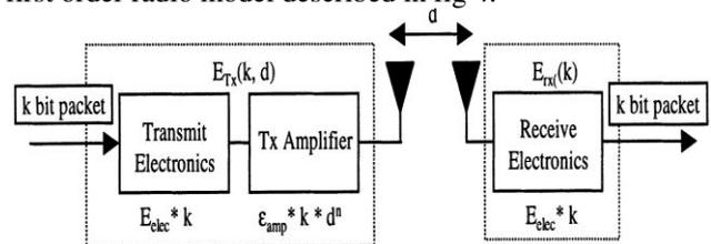
Fig4: Radio energy dissipation model
