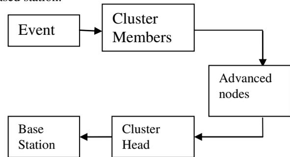
Fig. 3: Data propagation in WSN
