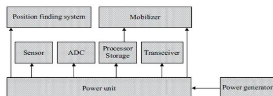
Fig. 2: Sensor node Architecture
